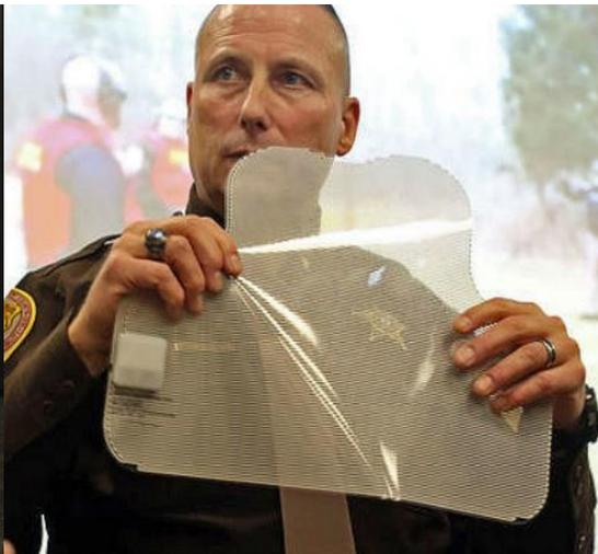
*Automatic Injury Detection (AID) Sensors can detect when an individual has been shot, stabbed or injured by shrapnel from an IED even if the wearer can be totally incapacitated; featured in this video from Montgomery County, VA Sheriff's Office.)*
