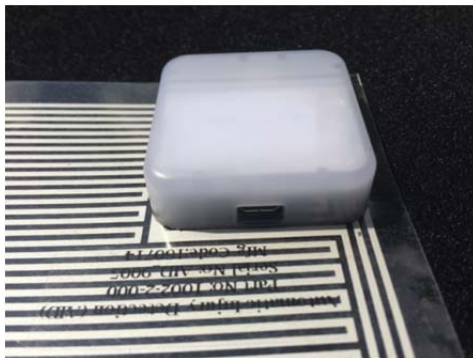
Figure 2: AID Communication Module Attached to Sensor Panel
