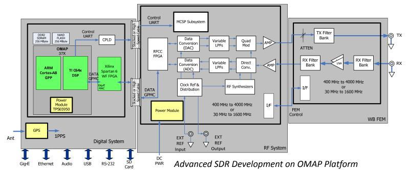
The TI OMAP platform supports development of waveforms and applications on Linux or Android operating systems
