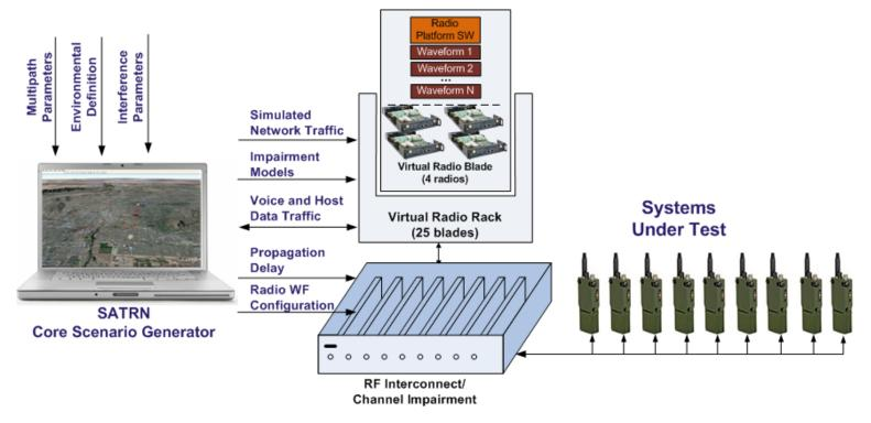
SATRN VRE: Create a Virtual RF Environment for realistic testing of large networks
